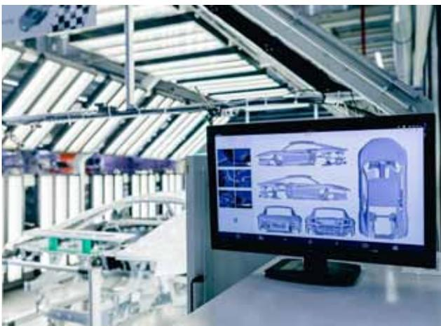
Assisted by artificial intelligence, a new light tunnel in the assembly line at Böllinger Höfe detects even the tiniest irregularities in finished vehicles.
