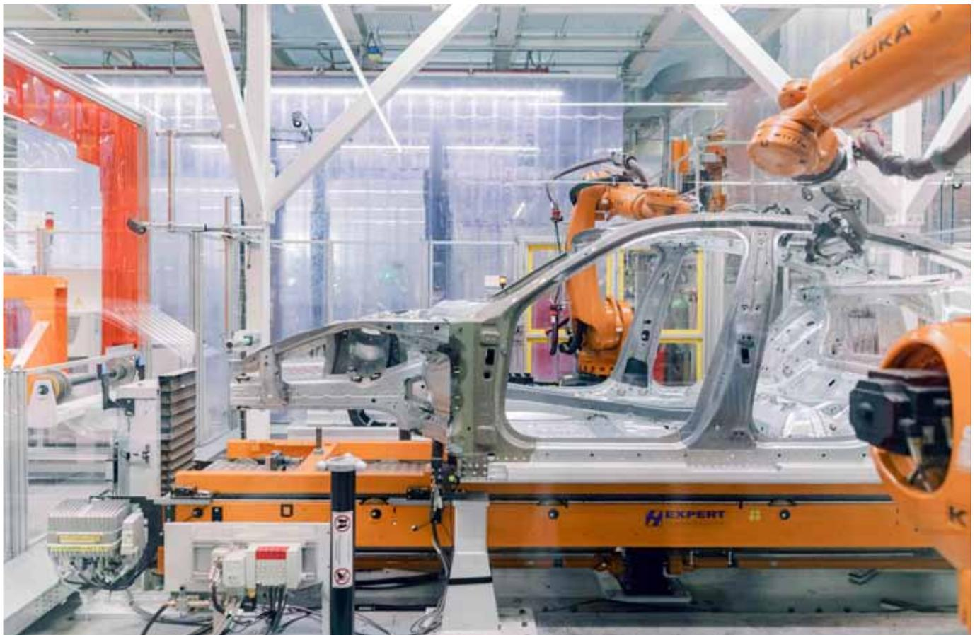
*The construction line for the Audi e-tron GT body uses correlation-free measuring techniques that, for example, perfect the dimensional accuracy of gap measurements.*
